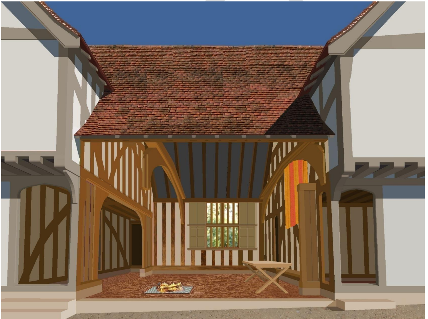
A cutaway reconstruction drawing of 4 Silver Street showing the interior of the open hall in the medieval period. The base of the original hearth was discovered in 2020 as well as fixings for a fabric wall hanging.
