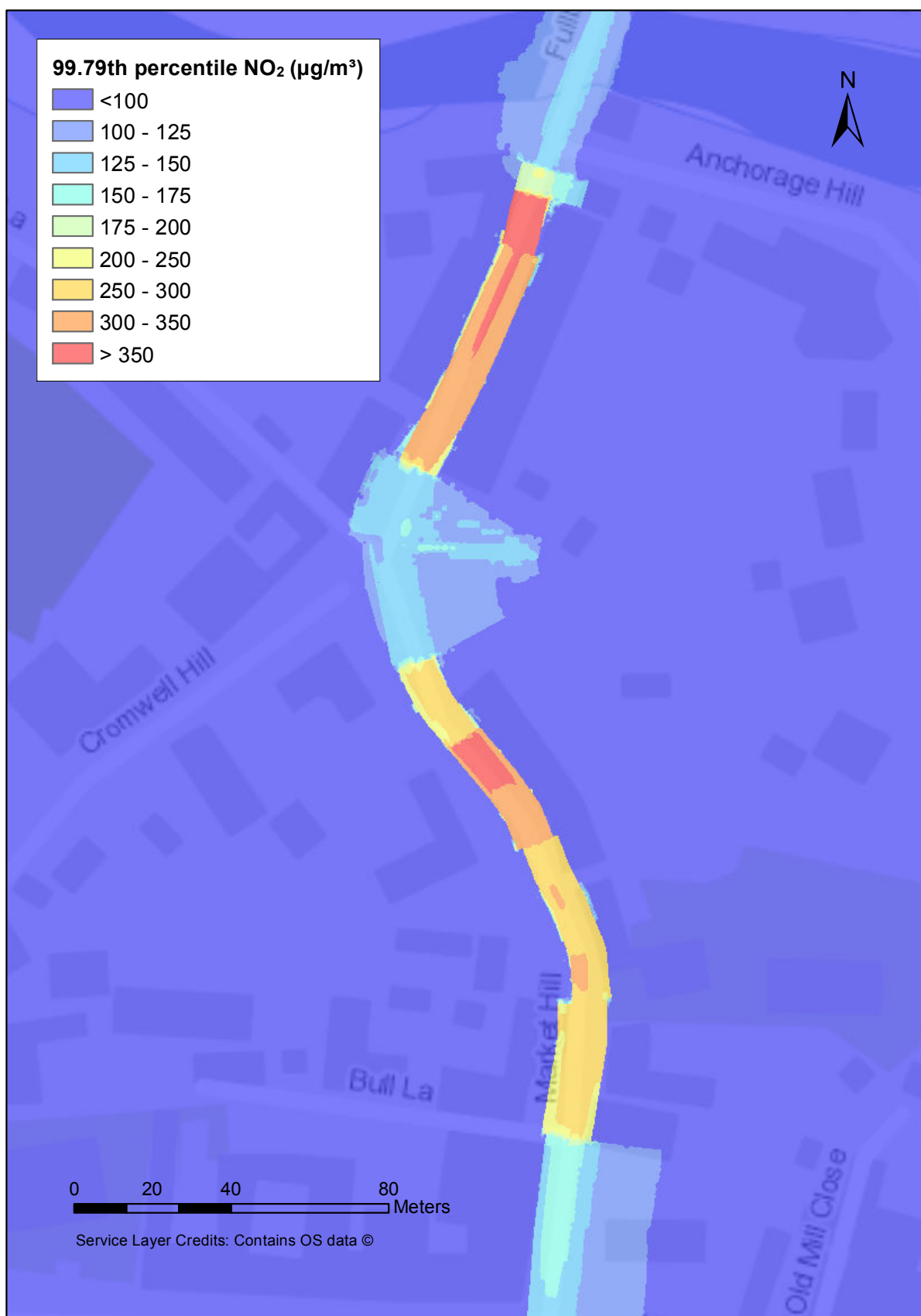
Figure 8.3: Modelled 99.79 th percentile of hourly average NO 2 concentrations (µg/m 3 ) along Market Hill Maldon
