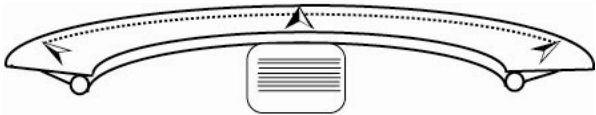
*The sketch above shows a stainless steel or brass plate to be attached to the outside of the existing black rails. (See picture on page 1)*
