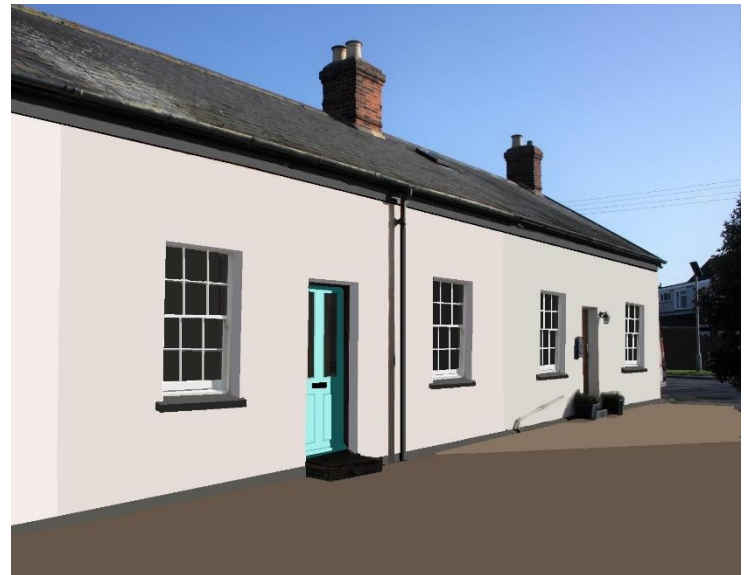
Fig. 43 – A mock-up showing how Nos 127 and 126 could be refurbished with sash windows, four-panel doors, and a resin-bonded-shingle surface to the lane.
